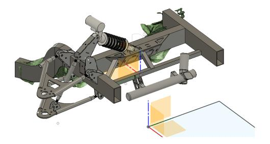
The suspension is fully designed and fabricated push/pullrod suspension setup. S10 knuckles are adapted in the front, with Acura knuckles in the rear. Each corner uses a hayabusa coilover and custom double A-arms. The control arm points were designed and validated using OptimumK suspension simulation and SolidWorks CAD and FEA.
