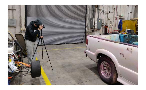
The first step in development was taking full 3d scans of the vehicle and frame components to aid in 3D CAD. The car was coated in multicolor chalk spray to create contrast and then pictured many times with a camera with low distortion lens. The photos were stitched together using Autodesk software to create 3D models to base the design off of.
