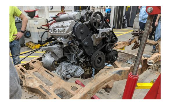
The powertrain for the S10 is a J32 and LSD 6 speed out of a 2007 Acura Type S. The engine is rigidly mounted in the bed of the truck driving the rear wheels, giving the vehicle a true mid-engined layout.
