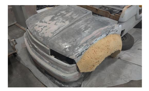
The S10 sports custom fiberglass bodywork molded off of the original front clip of the vehicle. The bed of the truck was skinned to be as light as possible. The truck is painted in a Spoon Sports inspired livery to pay homage to the Honda drivetrain.
