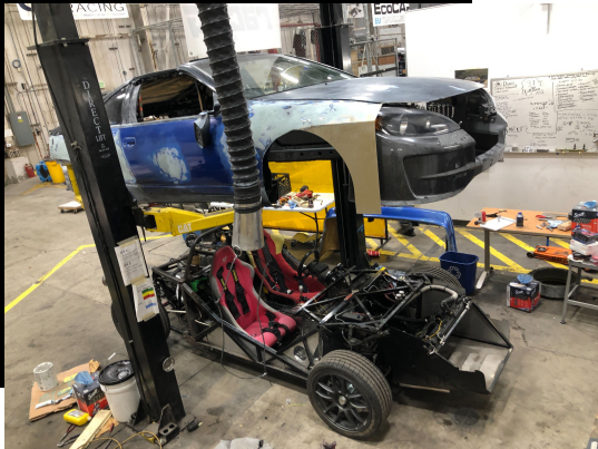
Test-fitting after bodywork
